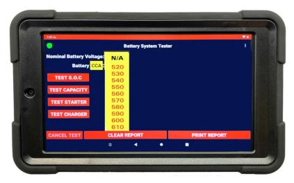
1. Press the TEST S.O.C button on the tablet to display the battery's state of charge.
